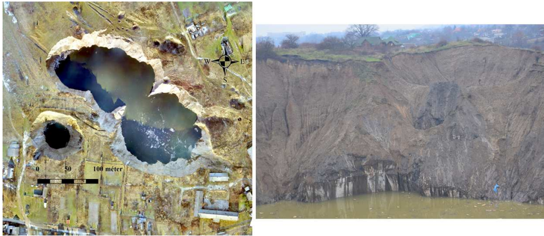
Figure 1. Pictures of some sinkholes in the Sotolvyno salt mining area (credit: Sándor Gönczy).
